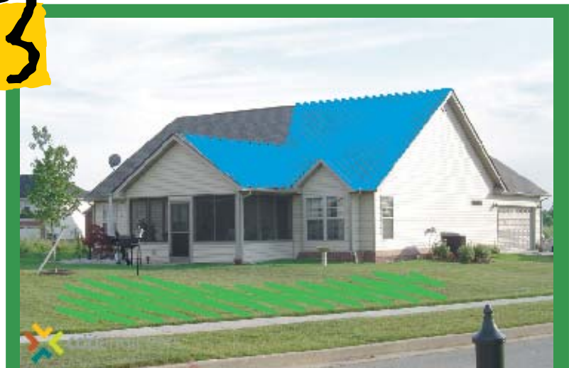
Calculate how much roof/yard area drains to the rain garden & the necessary rain garden depth
